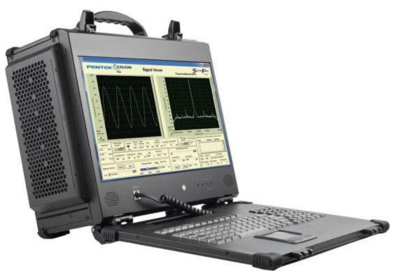
The Pentek RTR 2623 6GHz RF Sentinel intelligent signal scanning portable, rugged recorder has an integrated 6GHz RF down converter for real-time signal monitoring and detection that is user configurable.
